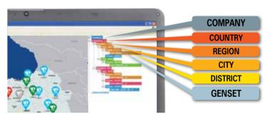
Besides, the capability of executing several adjustments optionally on the web interface increases the usability of the system. In case of need, many customizations are available such as regrouping genset sites on different basis.
